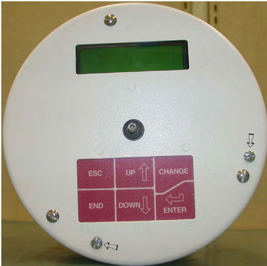
Figure 4-1 - Hydran 201Ti's User Interface
